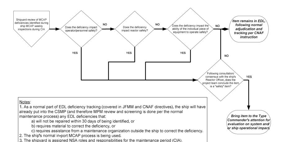
4. The shipyard's engineering and test engineering codes (246/2340) will review MCAP items identified from the weekly ship walkthroughs to determine if any items discovered require repair prior to the end of the inport maintenance period (CIA). Following consultation and consensus with the Reactor Officer/Commanding Officer, the item is brought to the attention of the Type Commander to schedule the repair
